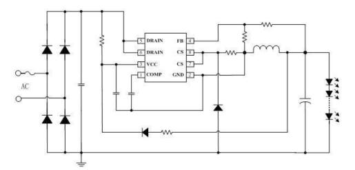
Figure 1. Typical application circuit for HW9616B
