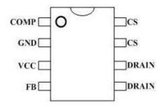
Figure 2. Pin configuration
