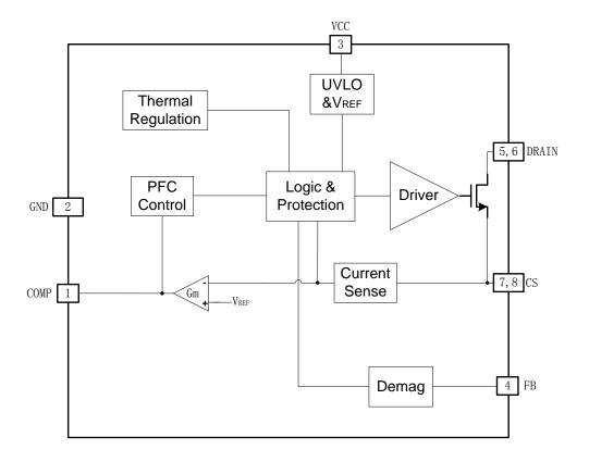
Figure 3. HW9616B Internal Block Diagram
